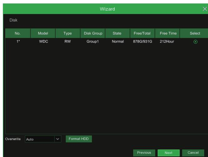
If the HDD is installed in the NVR for the first time, it must be formatted. Select the HDD and then click **Format HDD** button to format the HDD.
