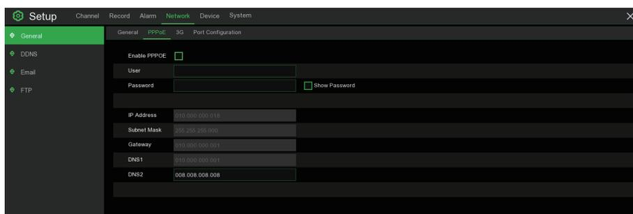
This is an advanced protocol that allows the NVR to connect to the network more directly via DSL modem. Check the "**Enable PPPOE**" box, and then enter the User name & Password of the PPPoE. Click **Apply** to save, system will reboot to active the PPPoE setting.
