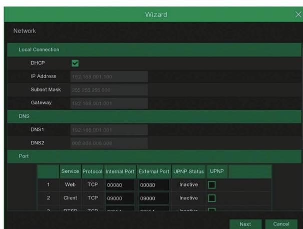
If you connect to a router allows to use DHCP, please check the **DHCP** box. The router will assign automatically all the network parameters for your NVR. Unless the network is manually addressed below parameters:
